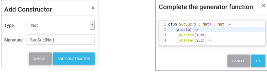
Fig. 8. Adding a constructor to a data type by completing a generator function template in the other decomposition.
